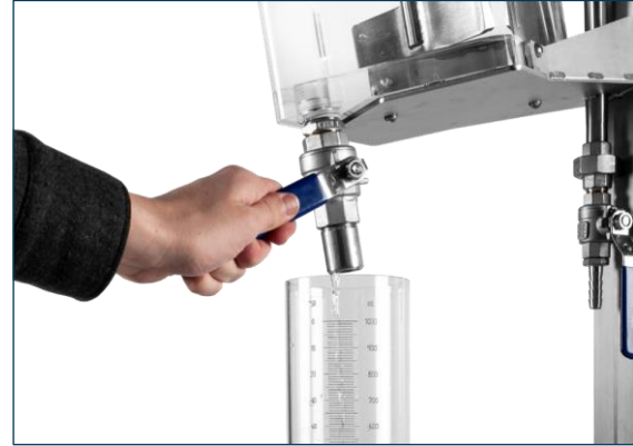
Sample taking via ball valve
