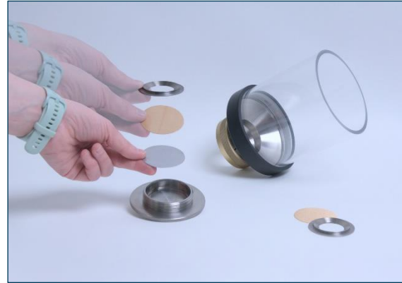
Insertion of wear plate and abrasion screen
